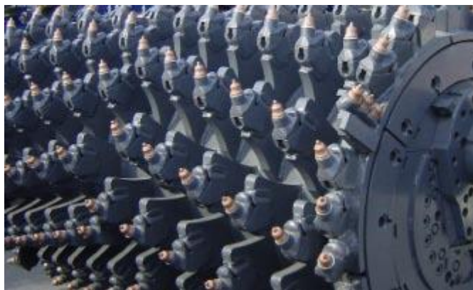
Figure 2:3 Cutting Tools on Milling Machines and Recyclers (Asphalt Academy 2009)
